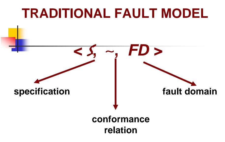
An implementation FSM *Imp* is *conforming* if *Imp* ~ *S* The objective of MBT testing – to detect each nonconforming  $Imp \in FD$
