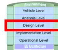
Design Level captures the concrete functional definition with a close correspondance with the final implementation
