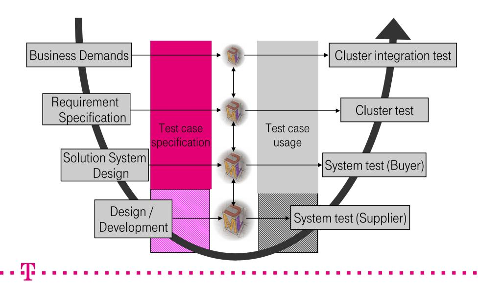
Interaction between system and test specification. Triggered for each milestone of the system specification.
