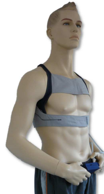
Textile-integrated ECG and wearable defibrillator
